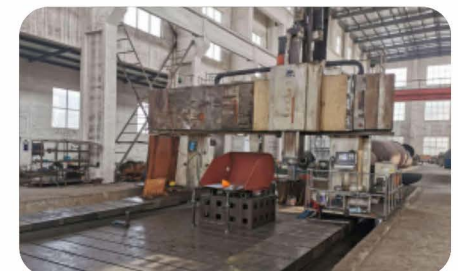
Gantry Portable CNC Boring-milling Machine 5 MetersX16 Meters
