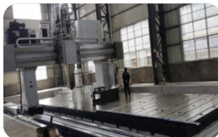
Gantry Portable CNC Boring-milling Machine 6 MetersX16 Meters
