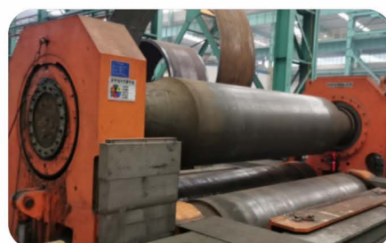
Rolling Machine 3.5 MetersX160mm thickness
